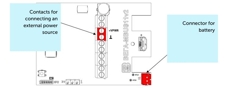
7. When the power is connected at the first time the device automatically switches to the "Active" mode and starts registration in the network. But if the device with connected battery or an external power has been switched to the "Storage" mode (by the pressing on the start button more than 5 sec) then you need to press the button to start.
